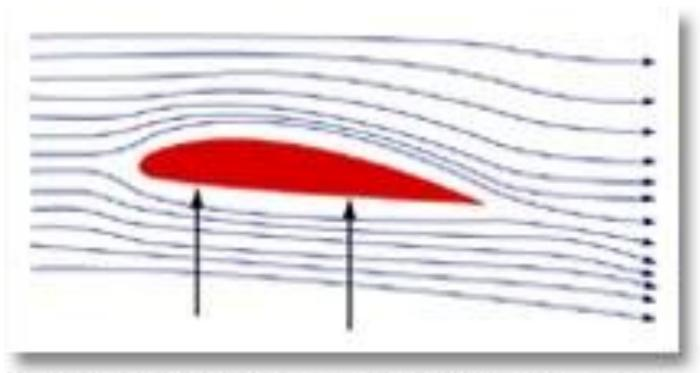
Cross section of an airplane wing. Air flows faster over the top than underneath, so exerts less pressure. Higher pressure air underneath the wing pushes it up.
