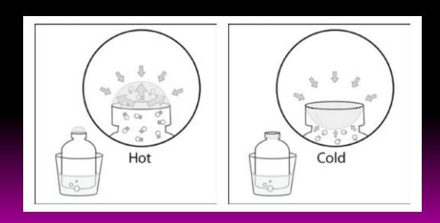
Heating/Cooling Gas in a Bottle
