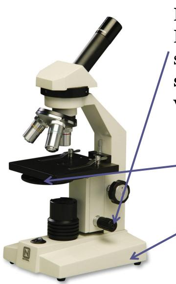
Fine Adjustment Knob – Moves the stage slightly to sharpen the image view
